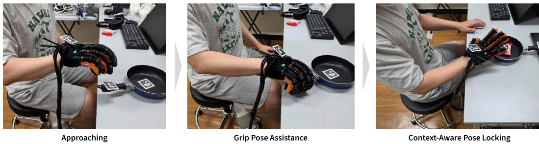
Fig. 3. Scenarios of Pose-based Human-AI Communication. Depending on motion trajectory toward the frying pan, different poses are assigned to assist or inhibit subsequent actions.
